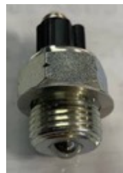
Neutral Switch (only provided for Manual transmission)
