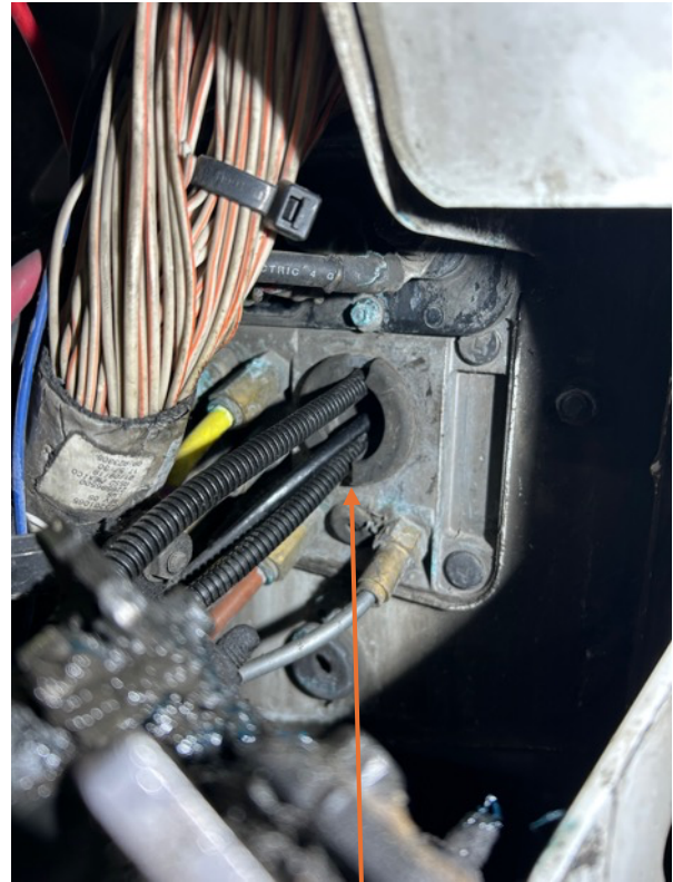
Use the larger pass-through if available. Cut out two notches in the grommet to run the Hood Switch & Buzzer harnesses
